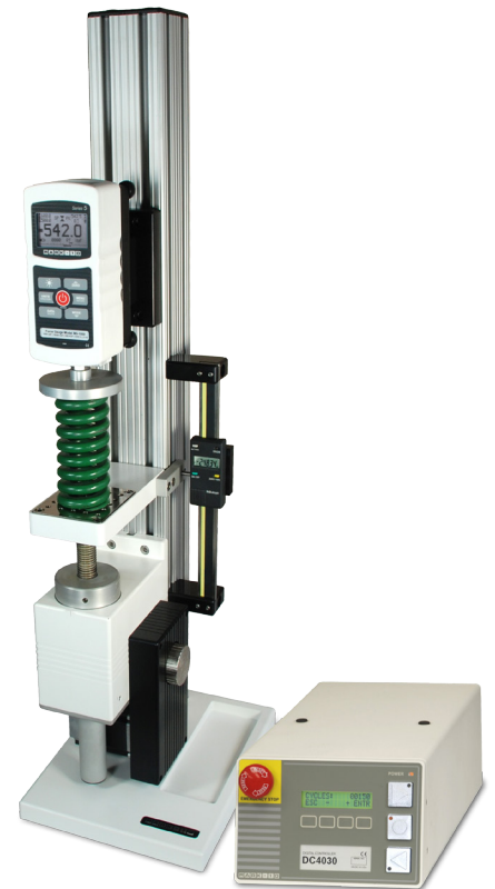
The TSFM500-DC is shown in a typical spring testing application, with Model M5-1000 digital force gauge and compression plate.
