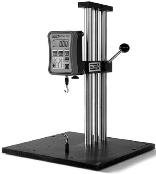
Wagner Force One™ FDIX Force Gage on FTK 100L Test Stand
