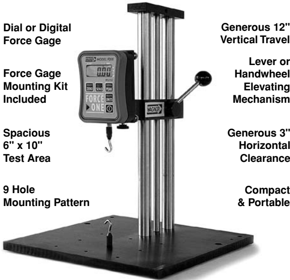
Basic FTK 100L Force Test Stand with FDIX Digital Force Gage
